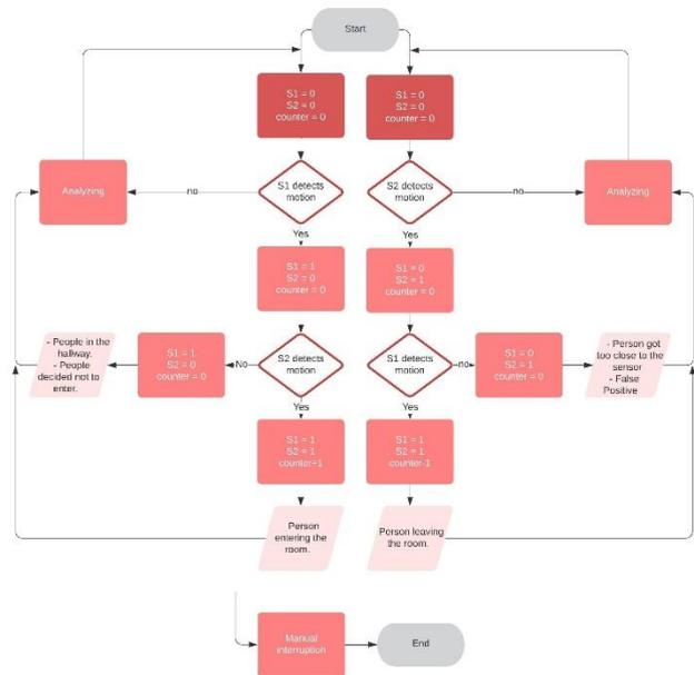
Figure 2. Flowchart of electronic people counting system using PIR sensors. Source: Author.
