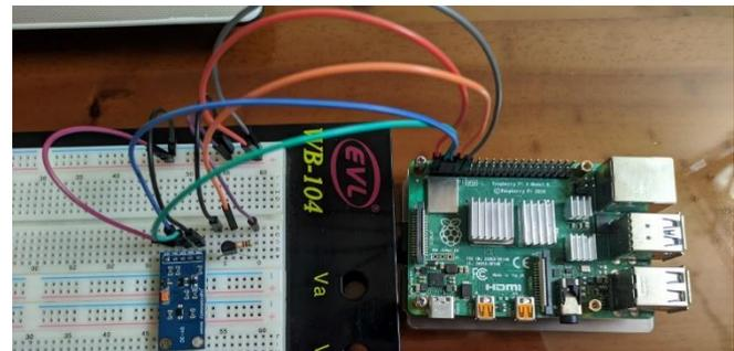
Figure 6. DS18B20 and BH1750 sensors connected to the Raspberry Pi 4. Source: Author.
